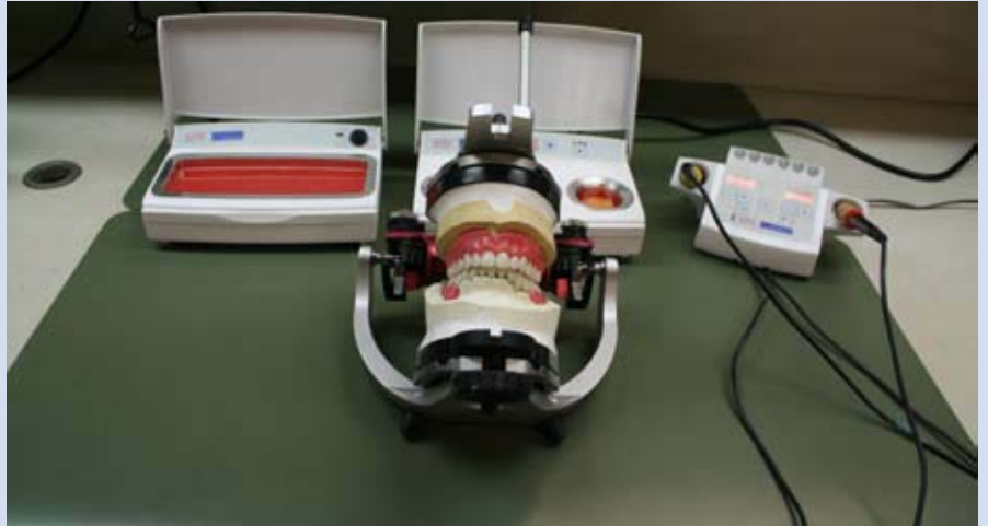
The ultimate waxing trio. Renfert's Waxprofi, the Vario E and the electronic waxing unit, the Waxlectric are essential for consistent temperature control of your waxing tips and most of all your waxes. Burnt wax loses its handling properties and becomes dirty which causes poor esthetics.
